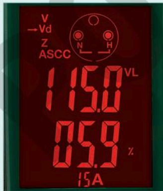
Display turns red when a problem is detected
